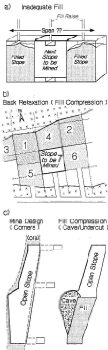
Figure 2.17.21: Limitations for use of Modified Stability Graph
