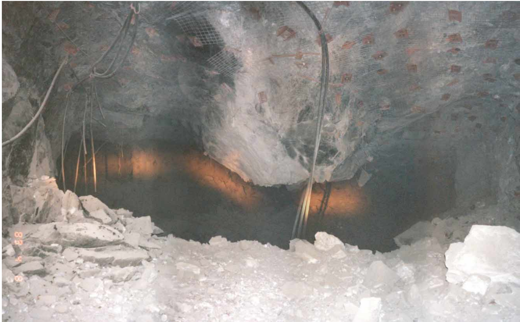
Figure 5a: Time-Dependent Ground Behaviour – BEFORE: SMALL OPEN STOPE IN TALC-CARBONATE ULTRAMAFICS
